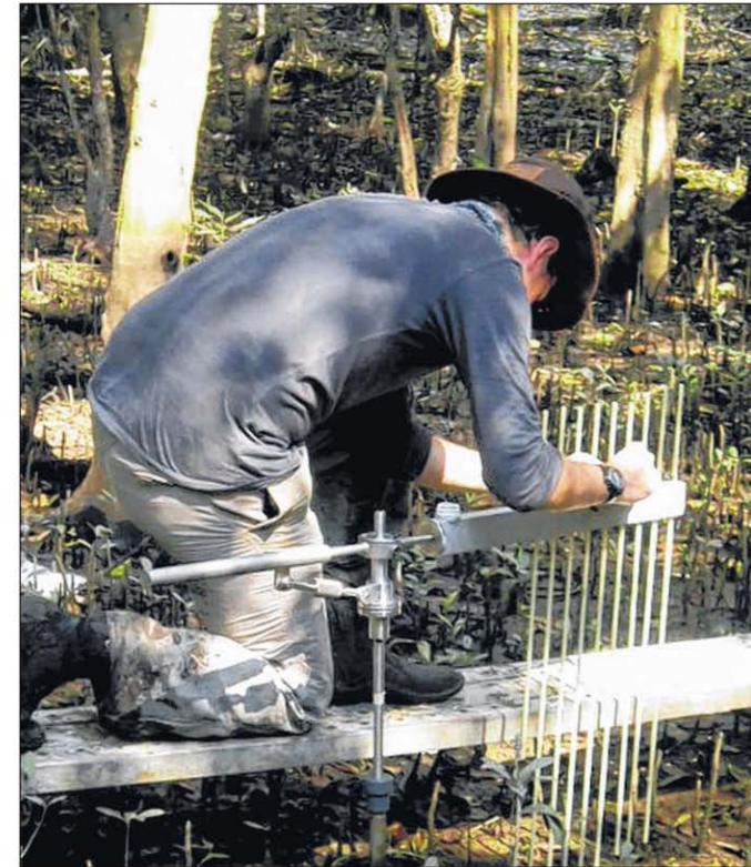
A rod surface elevation table being installed in a mangrove swamp.
